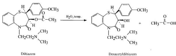
**Figure 1:** Degradation of diltiazem HCl to des-acetyl diltiazem
